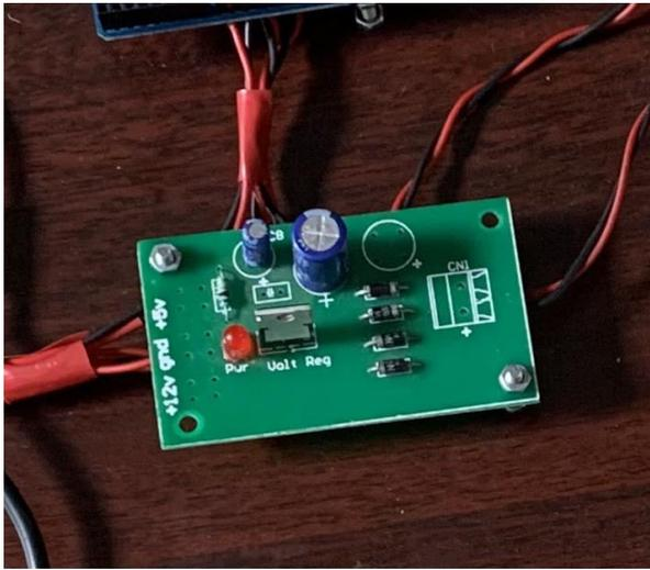
Figure 6: Power supply board
